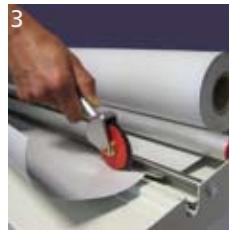
Cutting of Isogenopak® with a guide rail
